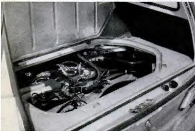
FOUR-CYLINDER ENGINE , under the floor in the three-door (station wagon) model, is fuel injected
